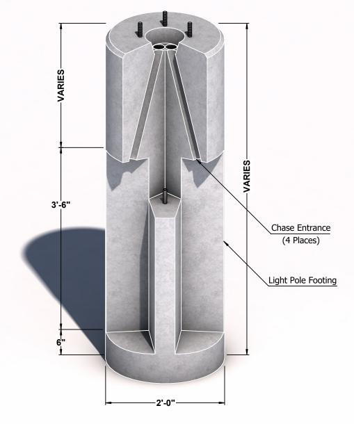
**Notes:** Light pole footing is set using lift plate secured to anchor bolt with nut. (2 Places)
